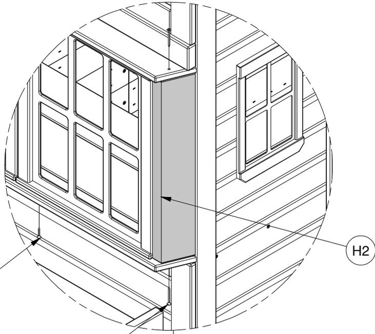
SCHRAUBE PFH 8x1 SD (4 PLCS) MITTLERE BOHRLÖCHER
